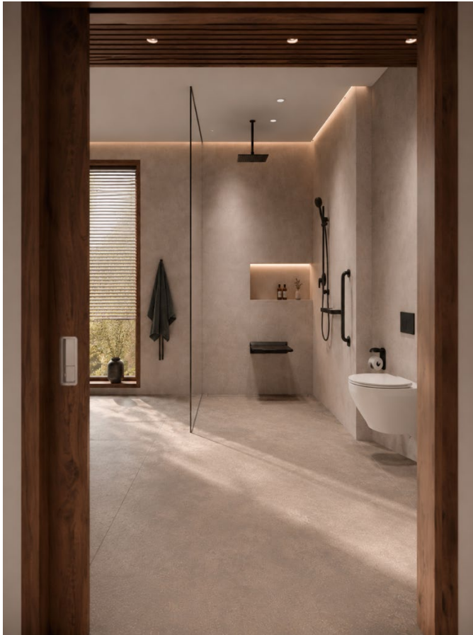
Figure 3 An adapted bathroom with level thresholds, accessible features like wet rooms and shower seats can be a very comfortable as well as enjoyable space without compromising on aesthetics
